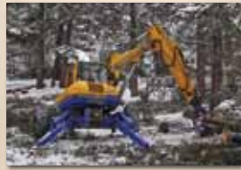
Here comes Spyderman! A low-impact Spyder hoe "walks" up winter hillsides to thin the forest, lifting whole trees without dragging them and avoiding damage to ground vegetation.
